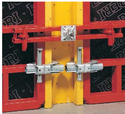
Levering corners make it possible to move the panel into position without using a hammer.
